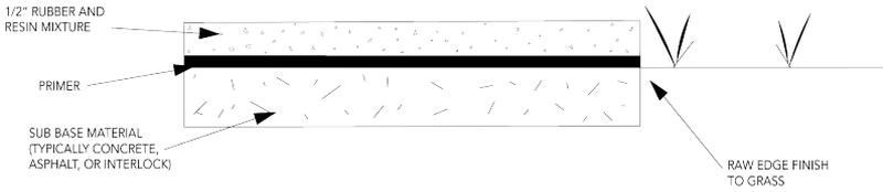
*Figure 2. Installation with raw edge.*
