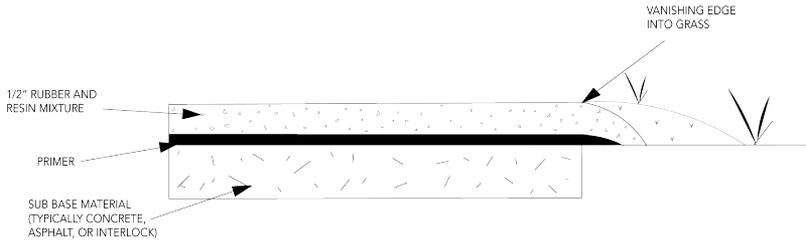
*Figure 4. Installation with vanishing edge.*
